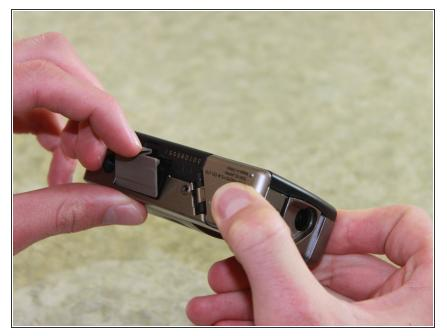
Locate the latch on the battery door marked by the word "BATT." Use your finger to pry it open.
