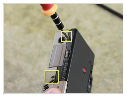
Locate and remove two 6.4mm screws on the bottom of the camera with a Phillips #00 screwdriver.
