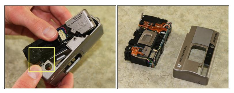
• Pull the front cover off of the camera by lifting the tripod tab over the tripod hole.
