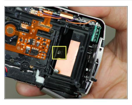
Locate and remove the 3.80mm screw inside the film compartment with the Phillips #00 screwdriver.
