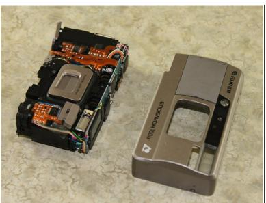
Pull the front cover off of the camera by lifting the tripod tab over the tripod hole.
