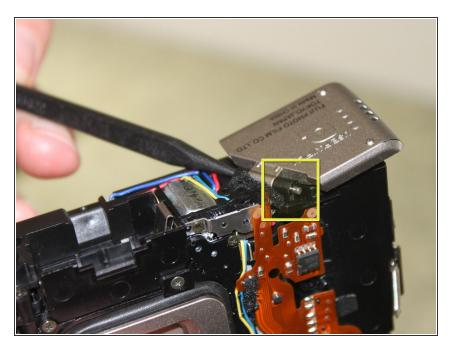
Push the pin from one side with the spudger until it comes out on the opposite side.
