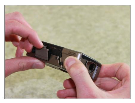
Locate the latch on the battery door marked by the word "BATT." Use your finger to pry it open.
