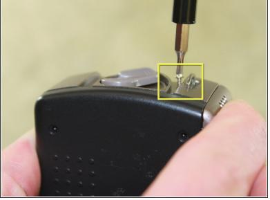
Locate and remove the 6.4mm screws located on either side of the camera with a Phillips #00 screwdriver.
