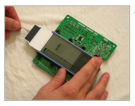
Slide out the screen from its case on the circuit board.
