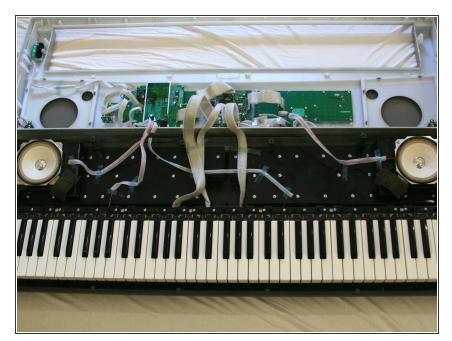
Locate the main circuit board - it should be toward the middle of the detached face plate.
