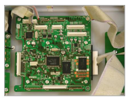
Completely remove the circuit board from the face plate.
