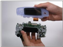
Using the tweezers, gently pull the ribbon from the logic board.
