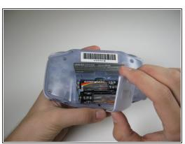
Take the battery cover off by releasing the locking tab and hinging the cover away.
