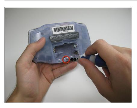
Remove bottom back panel screw with a Phillips #1 screw driver.
