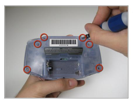
Remove the six back panel screws using a Tri-wing Screwdriver.
