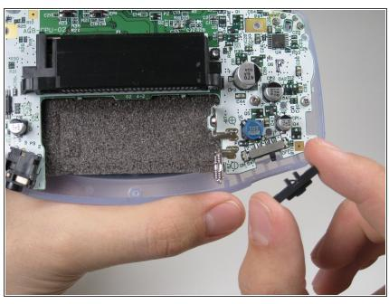
Remove the gray On/Off Switch by pulling up and away from the unit.
