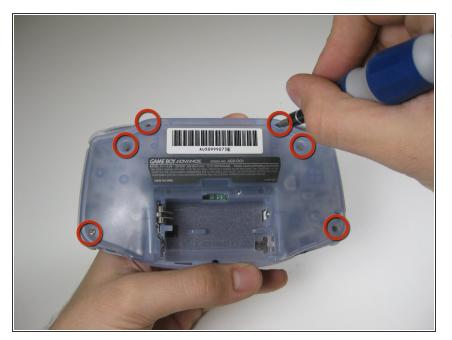
• Remove the six back panel screws using a Tri-wing Screwdriver.
