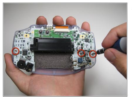
Remove the three screws on the circuit board with a Phillips #1 screw driver.
