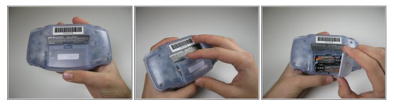
• Take the battery cover off by releasing the locking tab and hinging the cover away.
