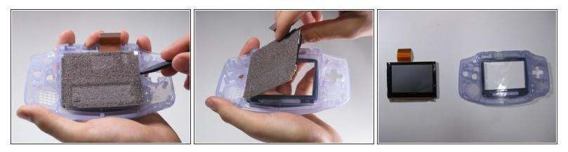
Use the spudger to lift the screen from the front panel. Place the spudger in the space directly left of the D-pad.
