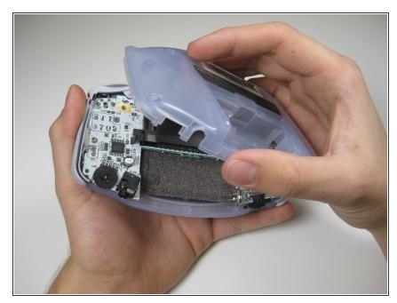
Remove the back panel by pulling away with one hand and the front secured in the other hand.
