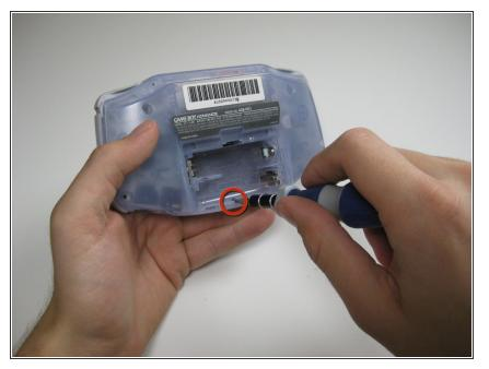
• Remove bottom back panel screw with a Phillips #1 screw driver.
