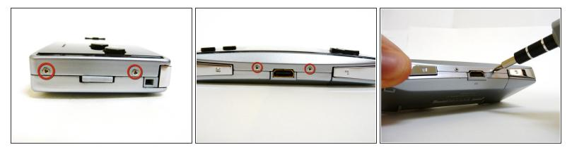
Remove the two tri-wing screws on the top of the Game Boy and the two screws next to the volume/contrast switch.
