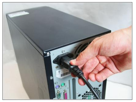
• Turn off your computer and remove the power cable by pulling it straight out of its socket.
