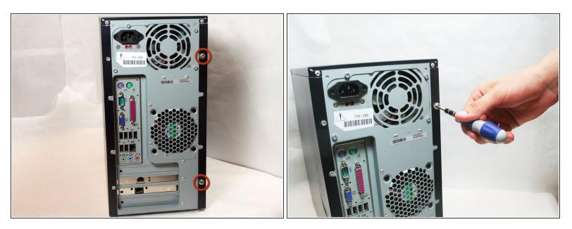
Remove the 2 Phillips #2 screws that secure the case door to the device.
