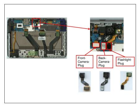
Carefully unplug the camera connectors from the mainboard and remove the cameras from their mounting. They may be attached by adhesives.
