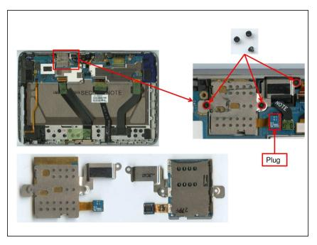
Carefully remove the 3 screws that attach the SIM-Card-Reader to the Mainboard. Detach the plug. remove the Card-Reader
