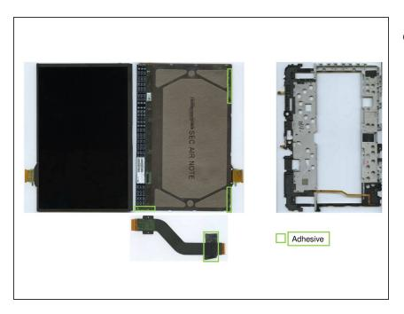
Once the front glass is removed, separating display unit and frame is a peace of cake. Just unplug the ribbon cable und detach it from the double sided adhesive that it is fixed with and pull off the display unit from the three adhesive areas. The display can be lifted off easily.
