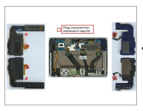
Carefully remove the speakers by loosening 2 plugs from each connector. Note that the speaker on
