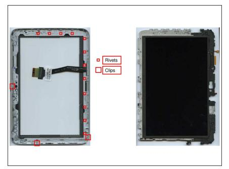
For the removal of the front glass, brutal force is required. The twelve clips that hold down the front glass must be (carefully) destroyed in order to detach the glass from the rest of the device.
