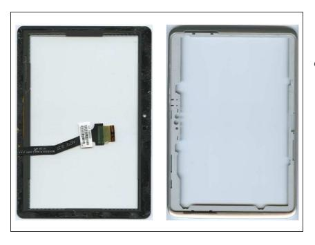
As glass and frame are bonded with strong adhesives, in order to separate both, a good lever is needed. The separation will likely leave scratches on both of the components.
