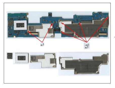
To remove the EMI-Shields, it is necessary to remove 4 screws from the back of the device. You can now lift off the EMI Shield. In order to remove the small Shield, 2 more screws need to be removed. After this the shields can be removed.
