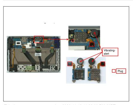
Carefully unscrew the scre that holds down the uSD-Card Reader, unplug the device. The Vibrating-Alert may be fixed with adhesives.
