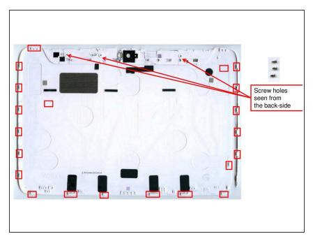
Remove 3 screws from below the camera cover and carefully open the 20 clips that are used to attach the back-cover to the main body.
