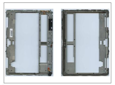
Frame and display unit are glued to each other like peanut butter and jelly. Pure force is required to disattach them. Use a lever. Difficult.
