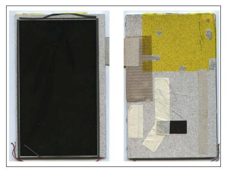
In order to separate display unit and front glass, much force is required to pry off both components
