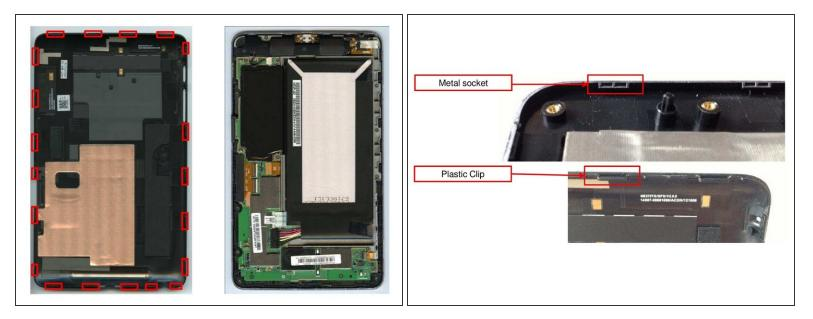
In order to open the device and remove the back cover a total of 20 clips need to loosened using a lever tool. This should pose no problem and leave the device undamaged.
