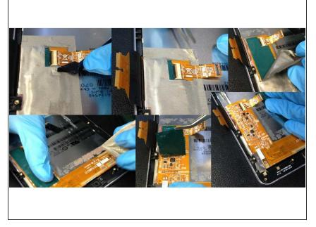
• The removal of the display unit will result in the destruction of the rest of the device. As the display is glued excessively to the rest of the device, it can only be removed using brutal force and a strong lever.
