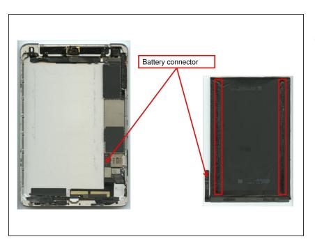
Once the display unit has been removed and the battery connector has been unplugged, the heat gun has to be used to warm up the adhesives that hold the battery fixed to the device.
