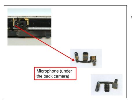
The microphone is located beneath the back camera of the device. It is fixed with strong adhesives and must be pried off with care.
