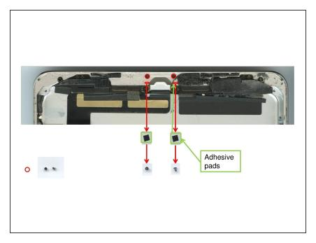
Close to the lightning connector, four screws need to be unscrewed using a #00 screw driver. Two of the screws are located underneath two adhesive pads.
