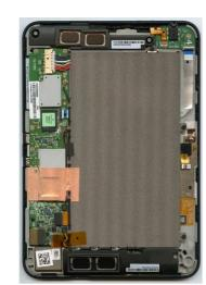
The back cover can be easily removed by applying a small lever tool to the edge of the device.
