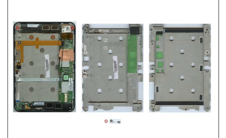
• By further removing two screws (#0) from the frame it is possible to separate the frame from the rest of the device.
