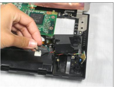
Pull the blue tab that holds the speaker chip and pull the chip out.
