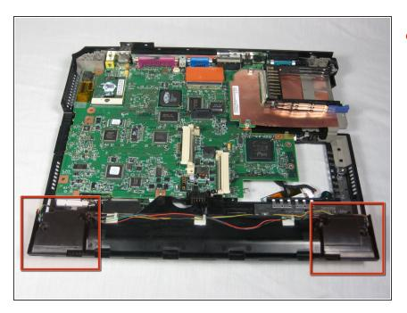
Locate the speakers on the bottom left and right of the ThinkPad A30.
