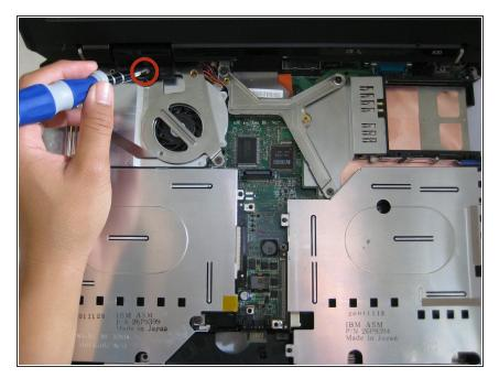
Remove the 5.6mm screw that holds the LCD to the upper case.
