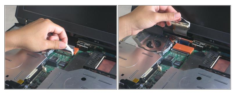
Pull out the white tab connecting the LCD to the motherboard.
