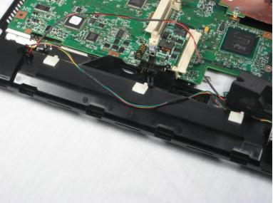
Remove the wires from the white tabs by lifting the black wire casing.
