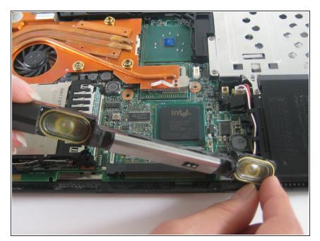
Lift the speakers out by starting with the left end and then unsnake the wires.
