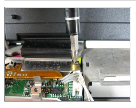
Remove a single screw from the metal plate that secures the display cable.
