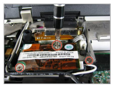
Remove the three screws holding down the modem in the upper left corner of the laptop.
