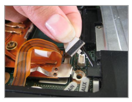
Unplug the trackpad's ribbon cable by pulling on the white plastic tab.
