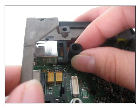
Remove the rubber microphone cover in the upper left hand corner by lifting up the gray metal frame.
