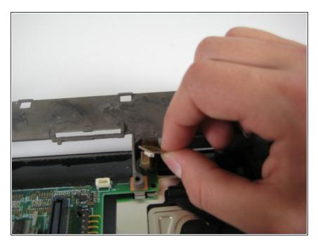
Disconnect the power connector from the motherboard.
