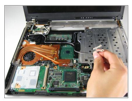
Carefully pull up the long antenna cables that were attached to the wireless network card.
