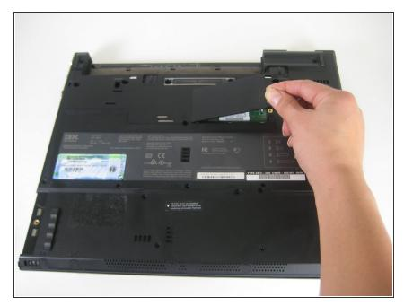
Remove the extra RAM cover, by lifting where the screw was and pulling out.
