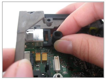
• Remove the rubber microphone cover in the upper left hand corner by lifting up the gray metal frame.
