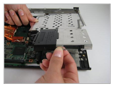
• Lift out the optical bay and HDD covers.
