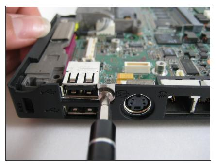
• Remove the single screw located next to the USB slots.
