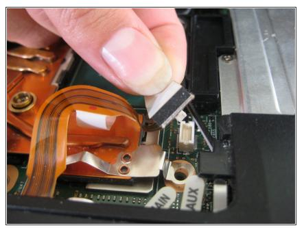
• Unplug the trackpad's ribbon cable by pulling on the white plastic tab.
