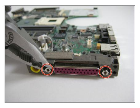
Using a nut driver or a pair of thin nose pliers, remove the two stand off screws next to the pink parallel port on the back of the computer.
