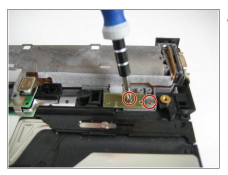
Remove the two screws in the upper right corner that secure the gray metal frame.
