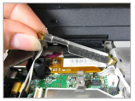
• Pull the metal plate away from the display cable.
