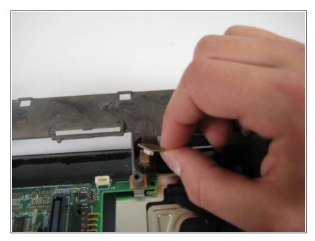
• Disconnect the power connector from the motherboard.
