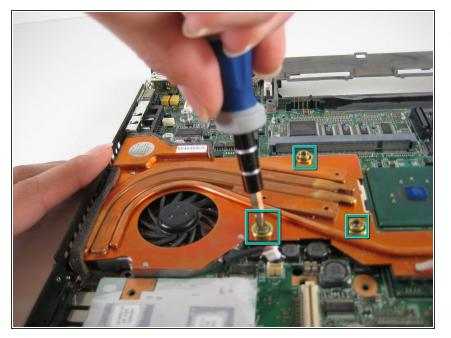
Remove the three screws on the fan.
