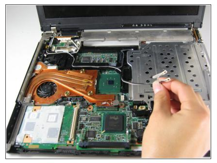
• Carefully pull up the long antenna cables that were attached to the wireless network card.
