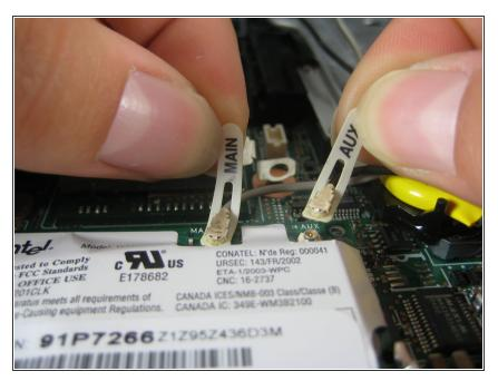
• Pull off the one black and one white coaxial cables by lifting the tabs labeled main and aux (for auxiliary).
