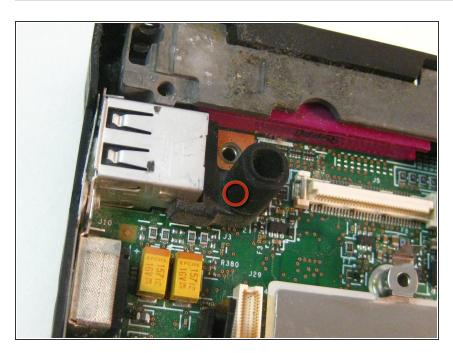
Then remove the small rubber piece covering the microphone.
