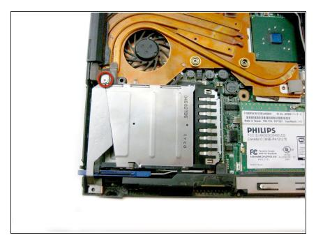
Unscrew the screw holding the port's bracket down.
