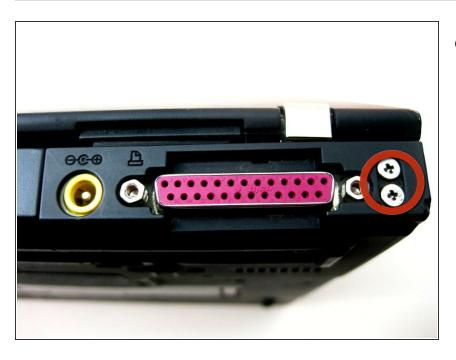
Unscrew the 4 screws on either side of the rear end of the laptop.
