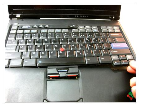
Flip the laptop over and open the display carefully - the keyboard, palm rest and bezel will be loose.
