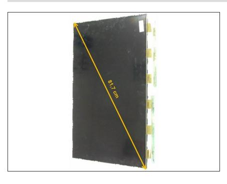
Carefully remove the already exposed LCD Panel.
