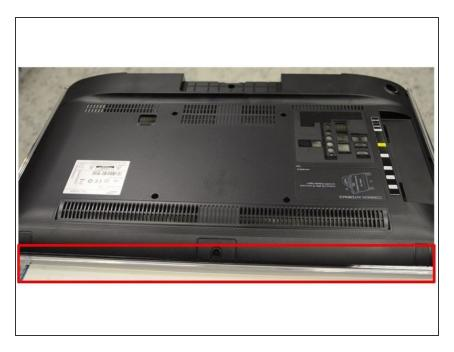
Note that two different type of polymers are molded together (red box). It is not possible to further separate them.
