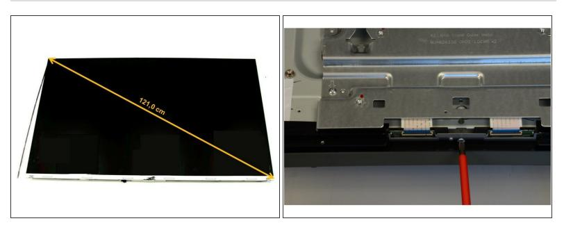
• Detach manually the two connectors of the back side and remove the LCD panel.
