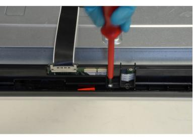
Using PH#2 screwdriver, loose eight screws of plastic and metal mountings used to protect different PCBs.
