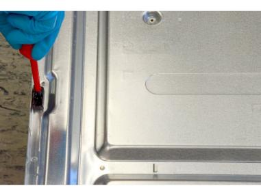
Remove plastic parts with PH#1 screwdriver and unscrew seven screws used to attach them to the metal-casing.
