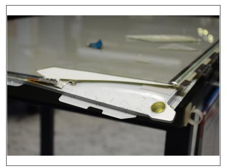
• The rest of the plasma panel is glued to a metal plate. Further disassembly not possible.
