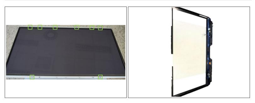
Remove the front glass frame from the dispaly unit. First, loose six PH#2 screws from the top and two PH#1 screws from the bottom of the frame.
