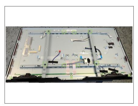
• Next, remove the metal plates using PH#2 screwdriver (thirteen screws).
