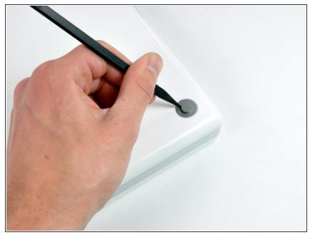
• Use a spudger or small flathead screwdriver to remove the three rubber feet from the lower case.
