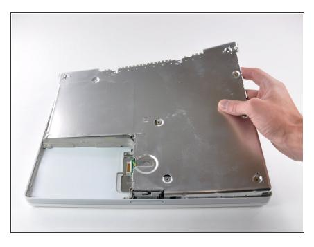
• Lift the bottom shield off.
