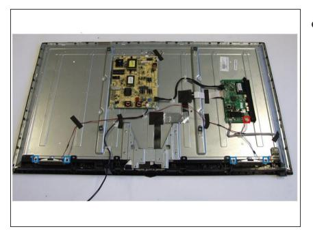
Manually pry open the connector (red box) and remove the speakers from their mountings (blue boxes).
