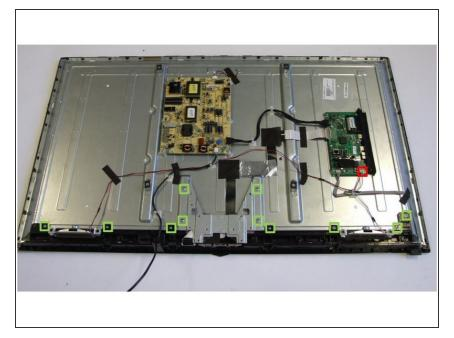
Using PH#1 screwdriver, loose eleven screws to separate metal and plastic parts.
