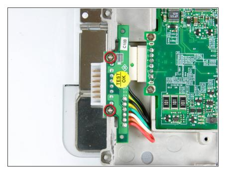
Remove the two Phillips screws securing the battery connector to the metal framework.
