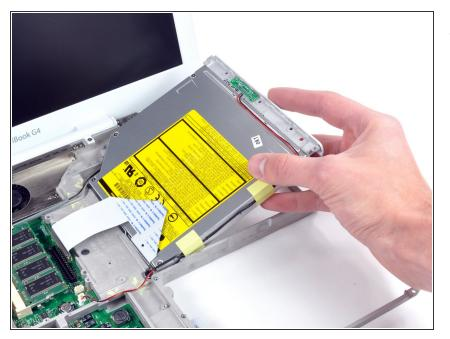
• Lift the optical drive from the metal framework.
