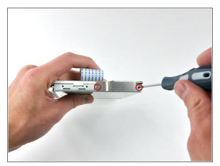
Remove the two Phillips screws securing the metal bracket and cable to the back of the optical drive.
