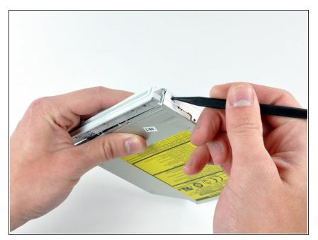
• Hold the optical drive on its side and depress the remaining tab to free the bezel from the drive.
