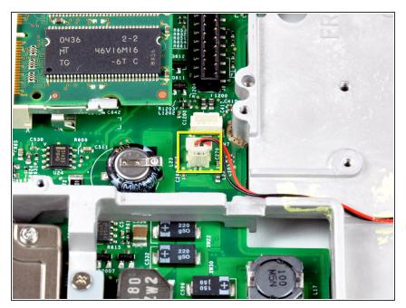
• Disconnect the Reed Switch board connector from the logic board.
