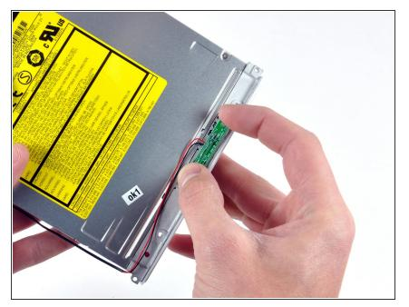
• Peel the reed switch board from the optical drive and set it aside.
