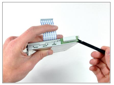
Peel the cable up from the top of the optical drive, removing tape as necessary, and disconnect its connector from the optical drive.
