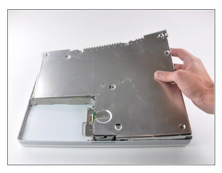
• Lift the bottom shield off.
