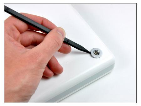
Use a spudger or small flathead screwdriver to pry up the three metal rings that housed the rubber bumpers.
