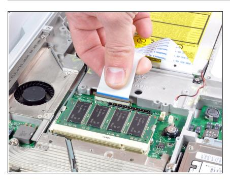
Release the optical drive ribbon clamp as described above. Slide the optical drive ribbon out of its connector.
