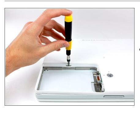
There is a slot on the wall of the battery compartment that locks the lower case in place. Use a small flathead screwdriver to pry out the slot's lower rim and pull up on the lower case to free the slot from the tabs holding it.
