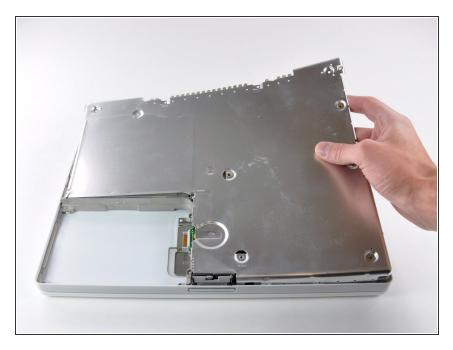
Lift the bottom shield off.
