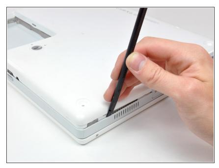
Continue to run the spudger around the front, right corner. There are two tabs on the port side of the computer, one near the front corner and one near the sound-out port.
