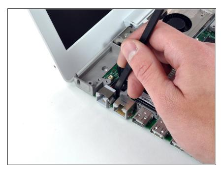
Wedge a spudger between the RJ-11 board and the metal framework and pry the RJ-11 board away from the logic board.
