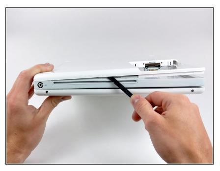
There are three tabs over the optical drive that must be released before the lower case can come off. Slide the spudger into the lower case above the optical drive and run it toward the back of the computer until you hear three distinct clicks.
