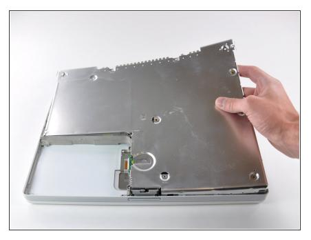
Lift the bottom shield off.
