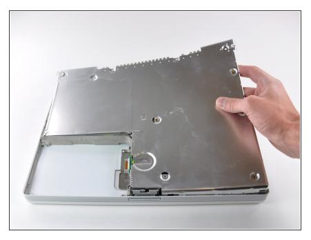
Lift the bottom shield off.
