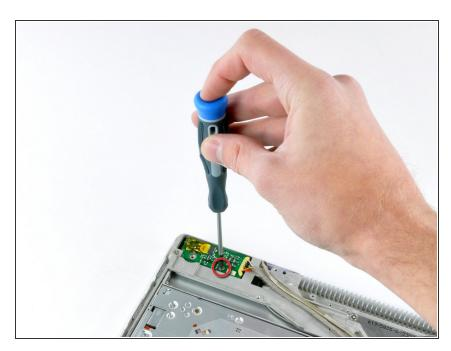
Remove the single Phillips screw securing the DC-In board.
