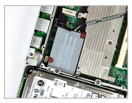
Remove the two 3 mm Phillips screws securing the AirPort card to the logic board.
