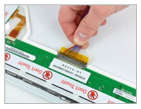
Disconnect the display data cable by pulling the cable away from the socket on the LCD.
