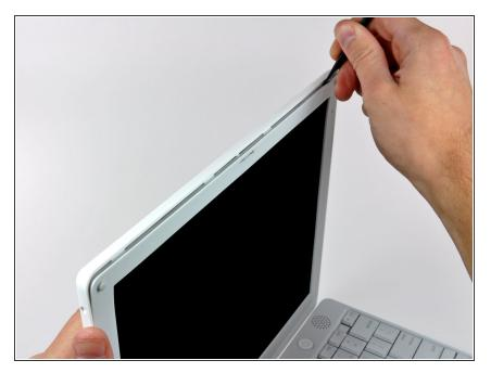
Run your spudger along the top edge of the front display bezel to evenly separate the two bezels.
