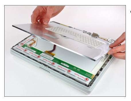
Carefully remove the thin steel LCD cover.
