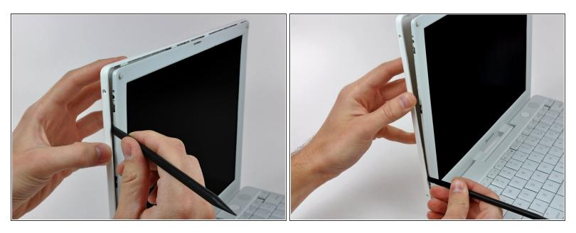
• Working down from the upper left corner, use the flat end of a spudger to pry the rear bezel away from the left edge of the display.
