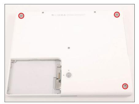
Remove the three newly-revealed Phillips screws.
