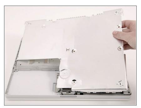
Lift the bottom shield off.
