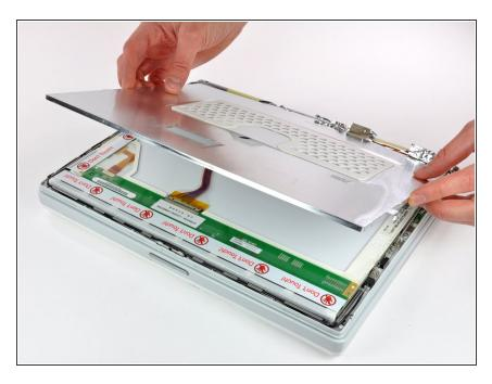
Carefully remove the thin steel LCD cover.
