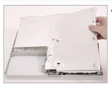
Lift the bottom shield off.
