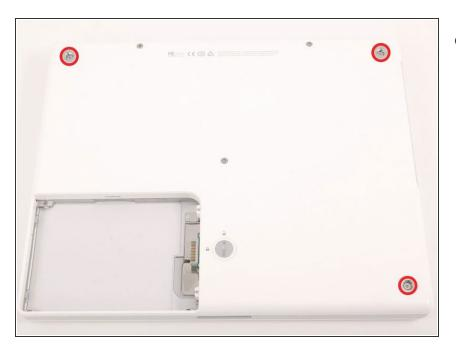
Remove the three newly-revealed Phillips screws.
