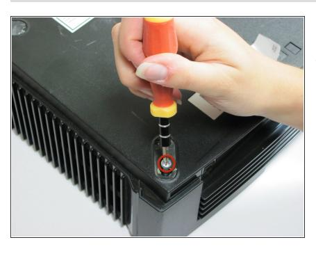
Remove the six T20 Torx screws securing the top cover to the bottom cover.
