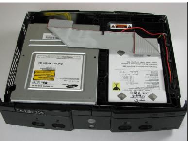
Once the bottom and top shells are no longer attached, carefully turn the Xbox right-side-up, lift and remove the top cover.
