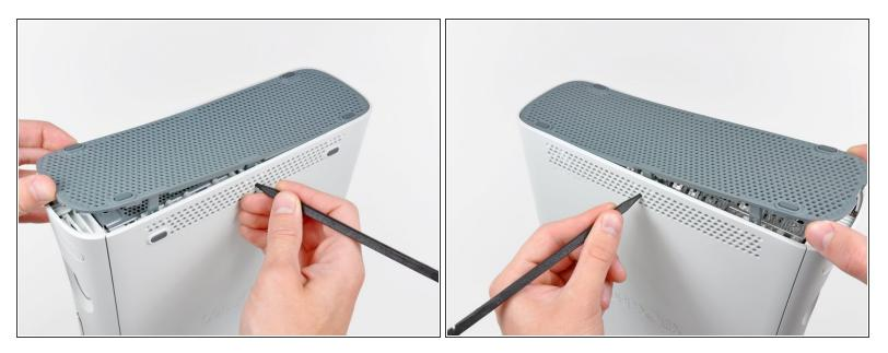
• Repeat the same process to release the two center clips on the bottom vent.
