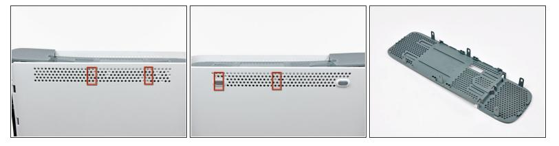
(i) In the next few steps, you will use the tip of a spudger or the finger of an Xbox 360 opening tool to release the clips along the left and right sides of the top vent. Their locations are highlighted in red.
