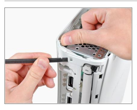
Insert the flat end of a spudger and pry upwards to release the last remaining latch located above the eject button.
