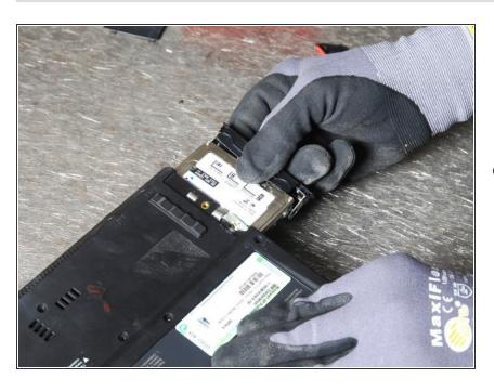
Remove all drives (HDD, CDD, etc.). If you cannot find the HDD, it is hidden most likely under the keyboard or under the top cover assembly. If you cannot find securing screws for the optical drive on the bottom, they are most likely under the keyboard.
