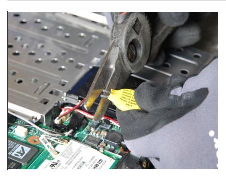
Remove the mainboard battery.
