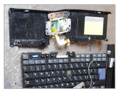
Lift the top cover assembly off the base and put it to the appropriate fraction.
