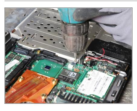
Remove all screws under the keyboard and cut/disconnect all cables.
