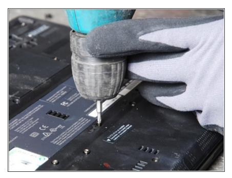
Remove all screws on the bottom of the laptop.
