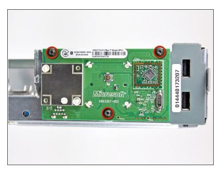
Remove three 5.6 mm T8 Torx screws securing the RF module to the metal chassis.
