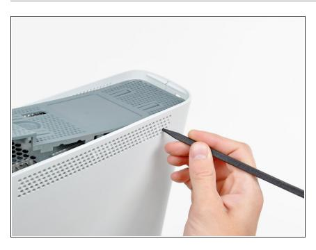
Use the tip of your spudger to release the clip on the top vent nearest the back of the Xbox's upper case.
