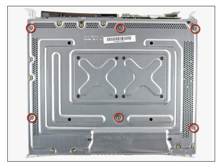
Remove the six silver 64 mm T10 Torx screws securing the upper case to the metal casing.
