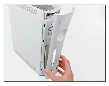
Remove the faceplate from the front face of the console.
