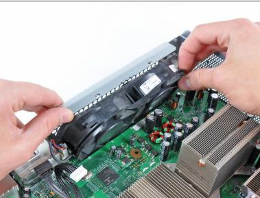
While lifting the metal chassis strip above the dual fans, pull the fans toward the center of the motherboard.
