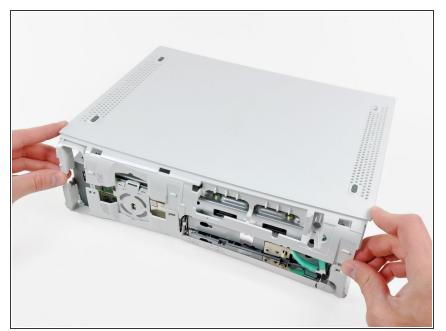
Slightly lift the front portion of the lower case to ensure that the latches in the front have been completely released.
